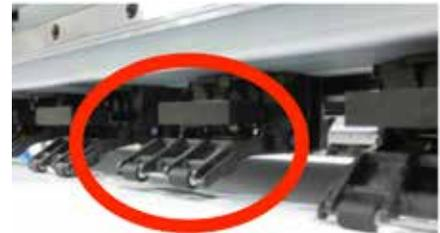
Operators can manually push down on the lever (above left) when the pinch roller is in the down position to raise it off the media (above right).
