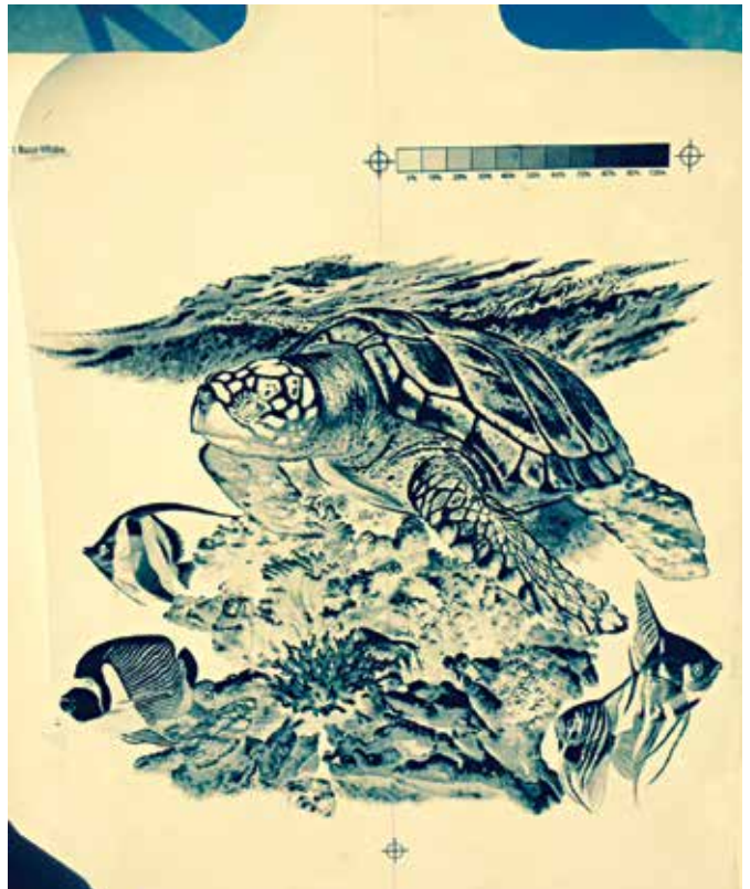
FIGURE B. Notice the grey scale in the top right-hand corner of the film positive. Exposing this grey scale on each screen for every color is a great way to visually inspect that all the halftone dots from the 5%-100% tonal range are exposed and washed out properly.
