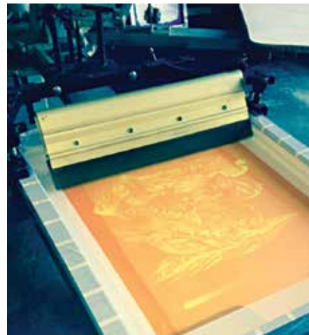
FIGURE A. Here, 20" x 24" OD static aluminum frames stretched to 20 N/cn were used to print the sea turtle. A 156-mesh was used for the white underbase and 230-mesh for the colors. Notice the amount of detail in the white underbase print.
