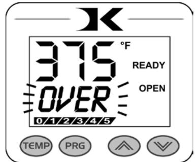
If the OverTemp alarm sounds, set the temperature to a higher value than the current actual temp. Wait 30 seconds and then reset the press to your desired temperature and Watch Carefully. Do not let the press rise to extremely high temps.
