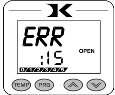
Once the temperature signal is restored (no longer broken, or plugged back into the control) the press will resume the temperature display, and start heating if necessary. If ERR persists, contact support.
