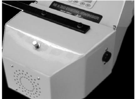
To interrupt the timing cycle, in order to do a quick pre-press or press for a shorter period of time than is set, simply press both black buttons together again. For emergency one-hand release of the air pressure, press the middle button on the front panel. **THE GREEN LIGHT MUST BE ON IN ORDER TO OPERATE THE PRESS.**
